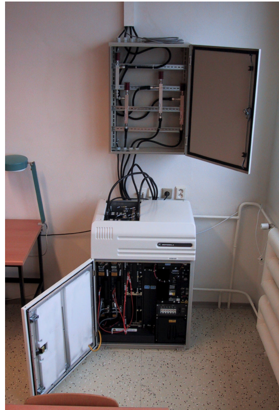
Fig. 1 Photograph of the base station MOTOROLA in the Laboratory of wireless and mobile communications.
