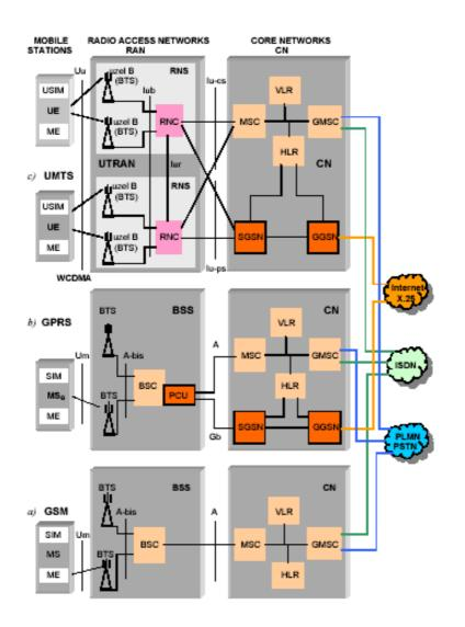
Fig. 2 Simplified cellular networks architecture: a) GSM; b) GPRS (with new nodes PCU, SGSN, and GGSN); c) UMTS (with new radio access network UTRAN)
