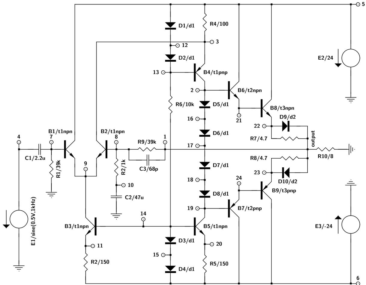
Fig. 3. AB-class power operational amplifier with wide spread poles and zeros on which all the reduction techniques have been compared.
