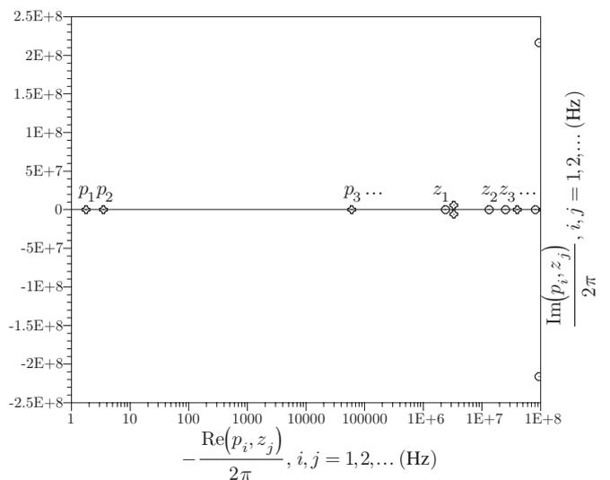
Fig. 2. Reduced poles-zeros (all divided by  $2\pi$ ) diagram of the linearized AB-class power operational amplifier.
