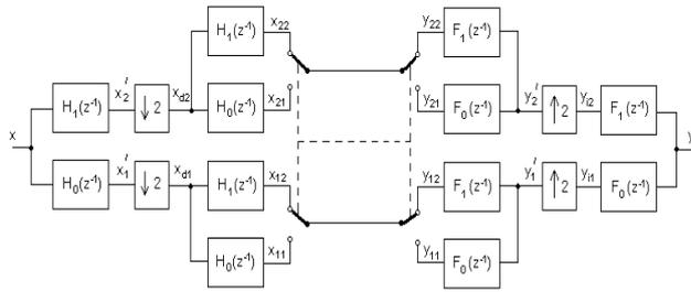
Fig. 8. Topology of the simulation model with tree-structured QMF.
