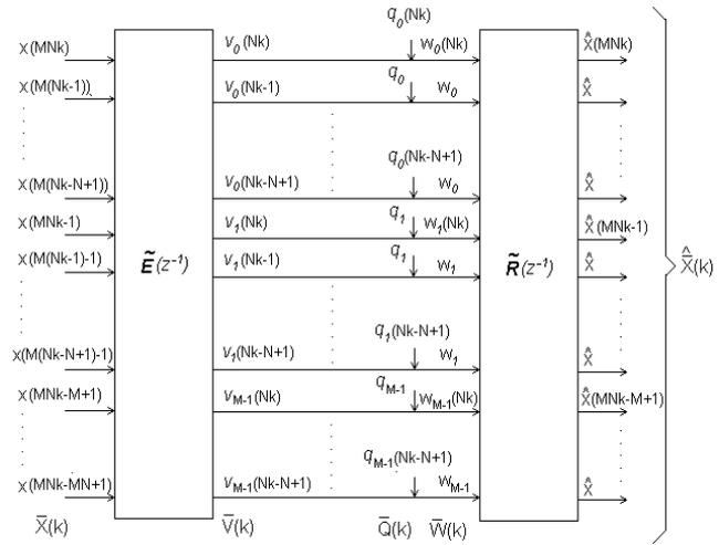
Fig. 2. Blocked polyphase representation of the filter banks.
