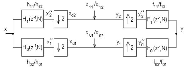
Fig. 6. Two-channel maximally decimated filter bank used for simulation.
