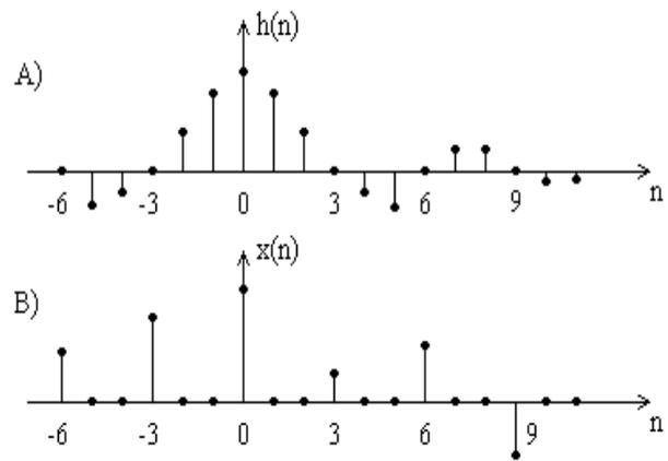
Fig. 3. Impulse response of the Nyquist- $M$  filter (A) and example of the input sequence (B).
