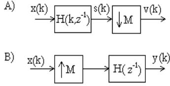
**Fig. 5.** Analysis filter cascaded with decimator (A) interpolator cascaded with interpolation filter (B).
