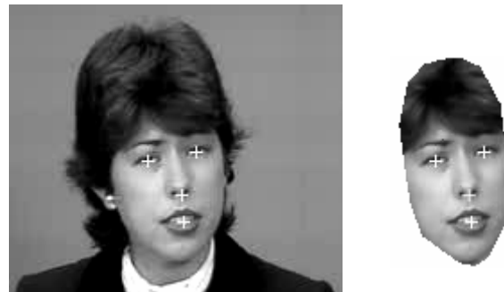
Fig. 3. A frame of videosequence Claire and the textured 3D model Candide perspective projected on the synthesized frame.
