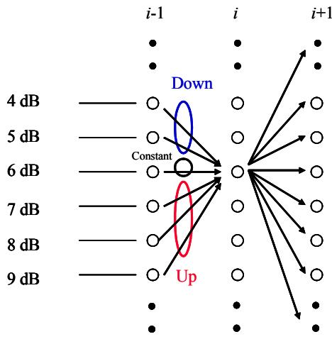
**Fig. 2.** DLR channel model as a discrete-valued 2<sup>nd</sup> order Markov chain. Grouping of transitions allows for a reduction of the number of transition probabilities.
