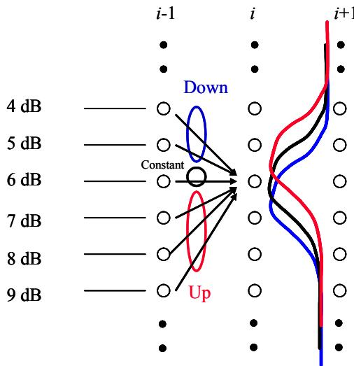
**Fig. 3.** DLR channel model: Description of the transition probabilities by Gaussian distributions.
