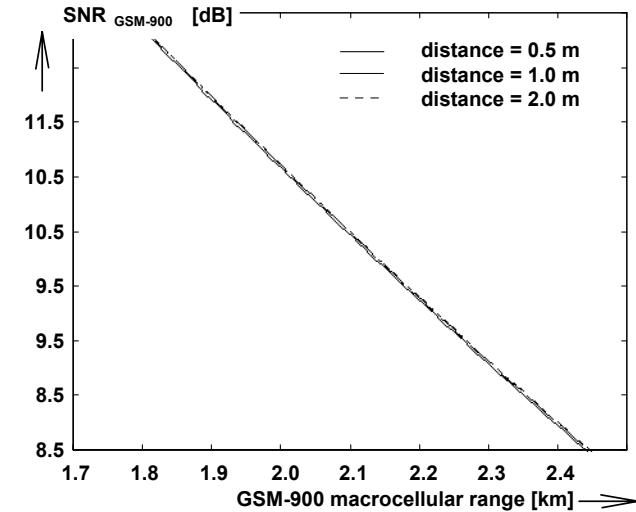
Fig. 4. GSM-900 SNR as a function of GSM-900 macrocellular range for 3 different distances between the UWB transmitter and the GSM-900 receiver when  $P_{UWB} = -100$  dBm/MHz.
