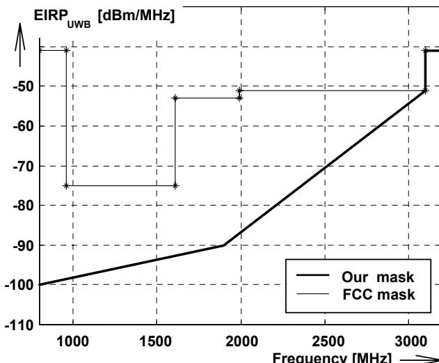
Fig. 5. The FCC and our recommended radiation masks.
