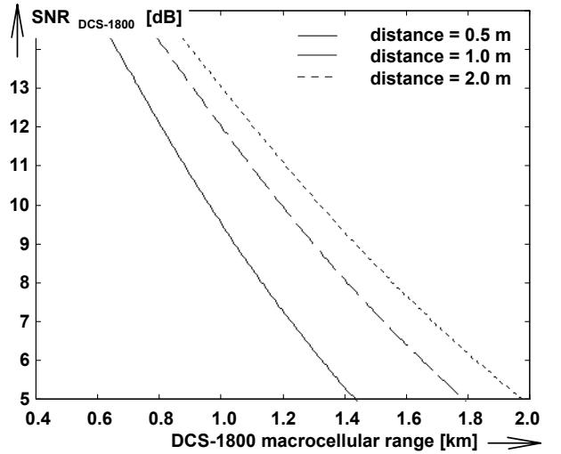
**Fig. 1.** DCS-1800 SNR as a function of DCS-1800 macrocellular range for 3 different distances between the UWB transmitter and the DCS-1800 receiver for  $P_{UWB} = -70$  dBm/MHz.
