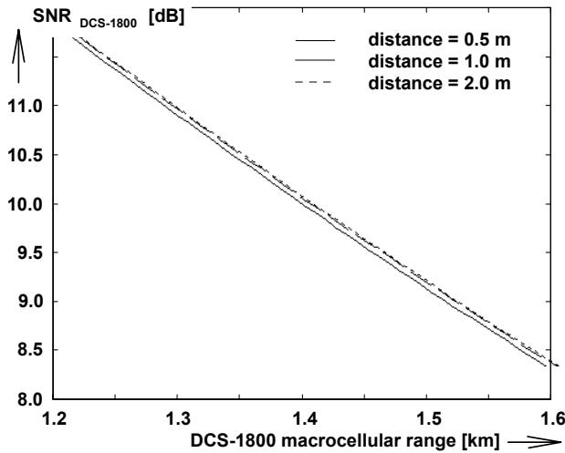
Fig. 2. DCS-1800 SNR as a function of DCS-1800 macrocellular range for 3 different distances between the UWB transmitter and DCS-1800 receiver when  $P_{UWB} = -90$  dBm/MHz.
