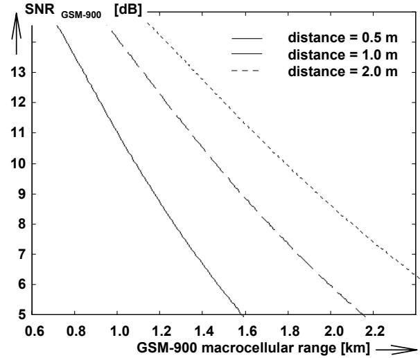
Fig. 3. GSM-900 SNR as a function of GSM-900 macrocellular range for 3 different distances between the UWB transmitter and the GSM-900 receiver when  $P_{UWB} = -70$  dBm/MHz.
