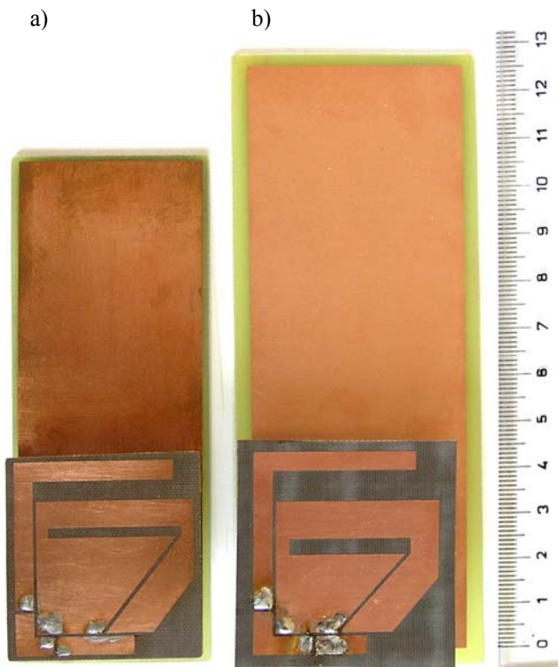
Fig. 14. Photographs of the realized antennas: a) the original one, b) the double-objective optimized one.
