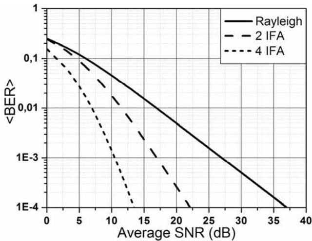
Fig. 3. The average BER versus average SNR for the reference (Rayleigh) and the 2- and 4- IFA receive diversity systems.
