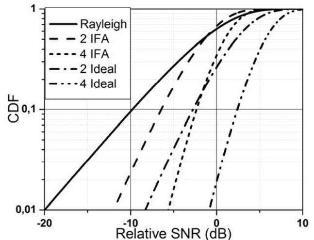
Fig. 2. The CDFs of relative SNR for the reference (Rayleigh), the 2- and 4- IFA and the ideal 2- and 4- branch receive diversity systems.
