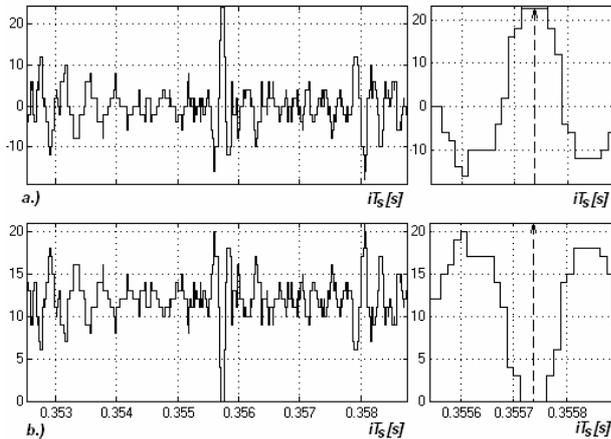
**Fig. 8.** (a) The result of the sample wise pattern correlation calculation (22),  $L_0=24$ ,  $E_b/N_0>25$  dB. Detailed scan of the correlation maximum. Its center is taken for symbol synchronization. (b) The result of equation (24) with the detailed scan of the correlation minimum.
