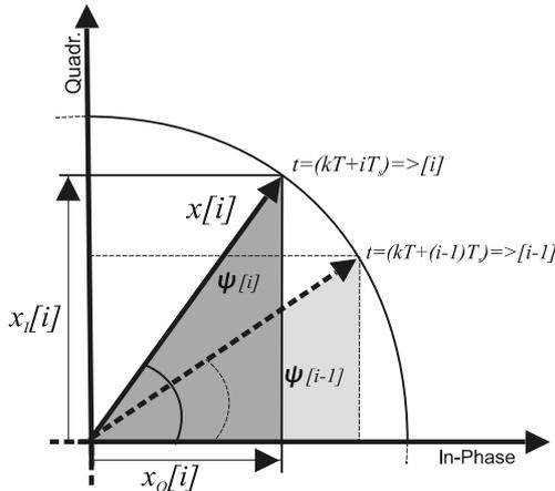
Fig.1. Vector representation of the received CPFSK signal.
