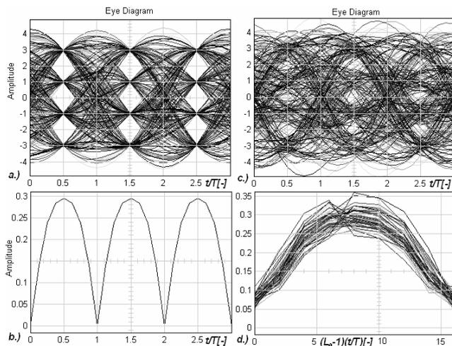
Fig.3. (a) Eye diagram of the demodulated 4-CPFSK signal  $m'[i-\tau]$  (Tx and Rx Root raised cosine filters employed with Rolloff=0.5) (b) Demodulated preamble signal  $m''[i-\tau]$  containing exact timing information. (c) Eye diagram of the demodulated 4-CPFSK signal with AWGN:  $E_b/N_0=15$  dB (-3dB Low pass Noise Bandwidth  $B_N=0.75R$ ). (d) Instances of the expectation function of  $\zeta(i)$  calculated according to (18).
