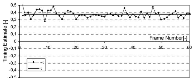
Fig. 6. Timing estimation variance over the received frames.  $E_b/N_0=10$  dB, preamble length  $L_0=16$ , 4-CPFSK, Tx root raised cosine filter employed with RollOff=0.5.
