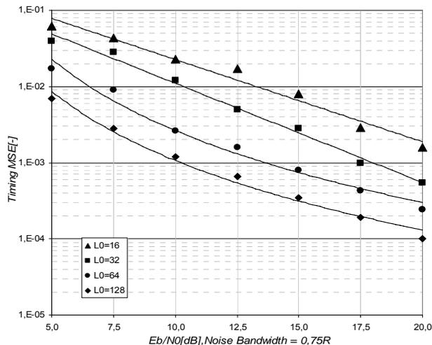
Fig. 5. Timing estimation MSE for different length of the NDA operation  $L_0=16,32,64,128$ .
