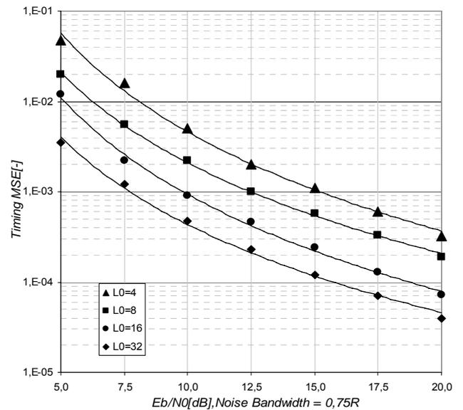
Fig. 4. Timing estimation MSE for different length of the preamble  $L_0=4,8,16,32$ .
