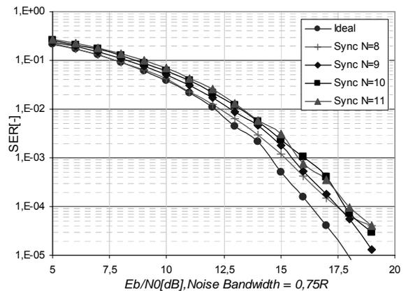
**Fig. 9.** Simulation results of the 4-CPFSK power efficiency with sample wise pattern correlation algorithm implemented.
