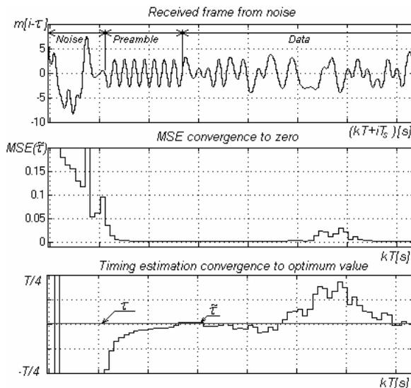
Fig. 7. Example of the timing estimate calculation over the receiving frame from band limited noise.  $E_b/N_0=25$  dB,  $L_0=16$ , 4-CPFSK, Tx and Rx root raised cosine filter employed with RollOff=0.5.
