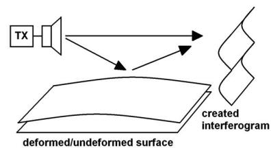
Fig. 1. Setup of the experiment for the scalar interferometric measurement of a deformation of a plain steel sheet.
