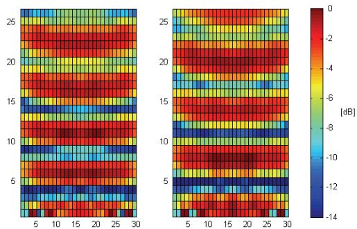
Fig. 2. Interferograms: plain steel sheet (left), deformed steel sheet,  $\Delta = 50$  mm (right). For the definition of the deformation  $\Delta$  see Fig. 3.
