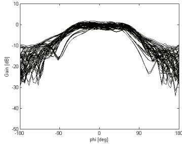
**Fig. 18.** Radiation patterns of all individual antennas in E plane in the vector antenna simulated in CST Microwave Studio.
