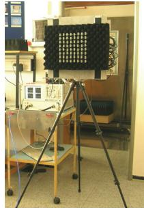
**Fig. 6.** Vector antenna matrix (8x8 elements) – general view.
