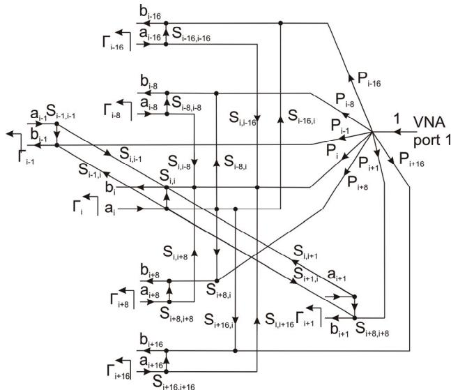
Fig. 10. Flow-graph – coupling effect between adjacent antennas.
