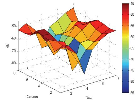
**Fig. 23.** Simulated measurement of an interferogram with interferometric fringes parallel to rows using the AM with real radiation patterns of individual antennas (E plane).
