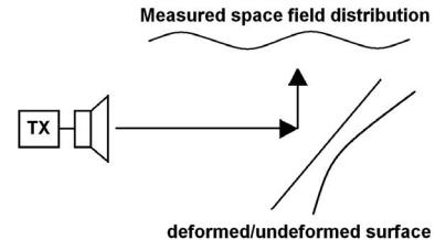
**Fig. 28.** Setup of the experiment for one-wave microwave interferometry.
