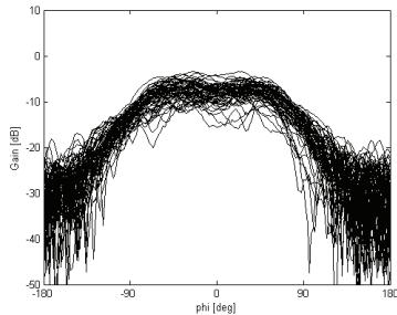
**Fig. 19.** Radiation patterns of all individual antennas in E plane measured in the vector AM using a microwave switch.
