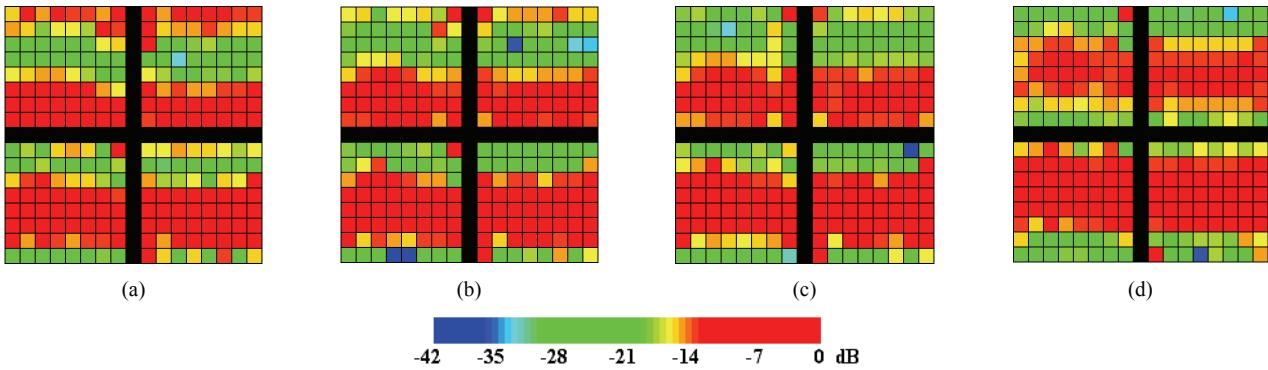
**Fig. 3.** Scalar interferometric measurement - experiment results at the frequency of 2.45 GHz. Amplitudes of the interferogram created by a plain steel sheet – without deformation (a) and with the deformation  $\Delta = 15$  mm (b),  $\Delta = 21$  mm (c),  $\Delta = 42$  mm (d). The deformation  $\Delta$  is defined as a height of the center of the deformed steel sheet in comparison to the plain undeformed sheet.
