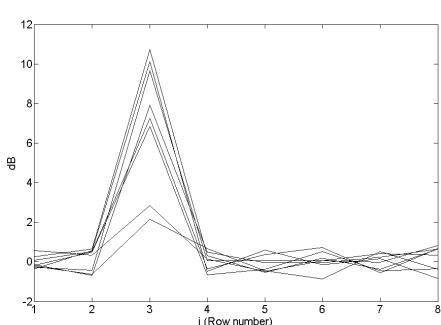
**Fig. 9.** Interferogram differences for simulated measurements based on properties of an ideal AM and properties of the realized and measured vector AM - 8 various columns.
