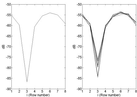
**Fig. 8.** Simulation - interferogram measured with the AM with no mutual coupling between individual antennas (left) and with mutual coupling - 8 various columns (right).
