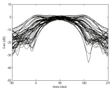
**Fig. 20.** Radiation patterns of all individual antennas in H plane in the vector antenna simulated in CST Microwave Studio.
