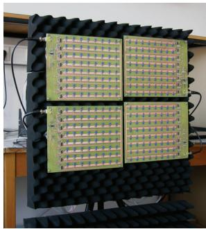
**Fig. 4.** Scalar antenna matrix (16x16 elements) - general view.
