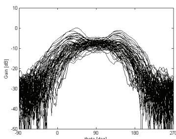
**Fig. 21.** Radiation patterns of all individual antennas in H plane measured in the vector AM using a microwave switch.
