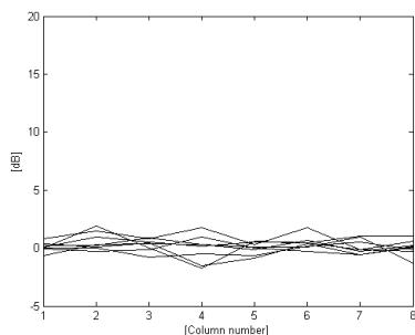
**Fig. 17.** Measurement error  $|P_i^M| - |P_i|$  (8 various rows).
