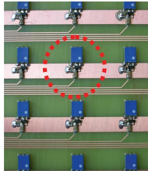
**Fig. 5.** Scalar antenna matrix (16x16 elements) - detailed view of a particular antenna with a RF diode detector.
