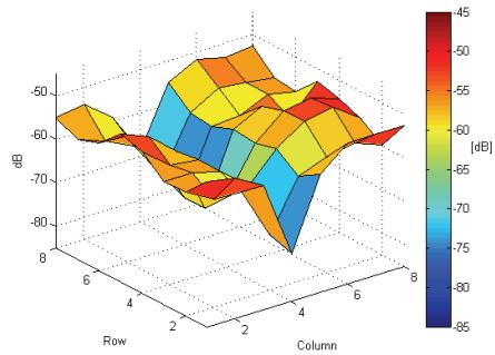
**Fig. 27.** Measurement of an interferogram with interferometric fringes parallel to columns measured using the real vector AM.
