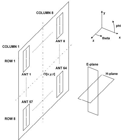
**Fig. 7.** Vector antenna matrix (8x8 elements) - indexing of individual antennas.
