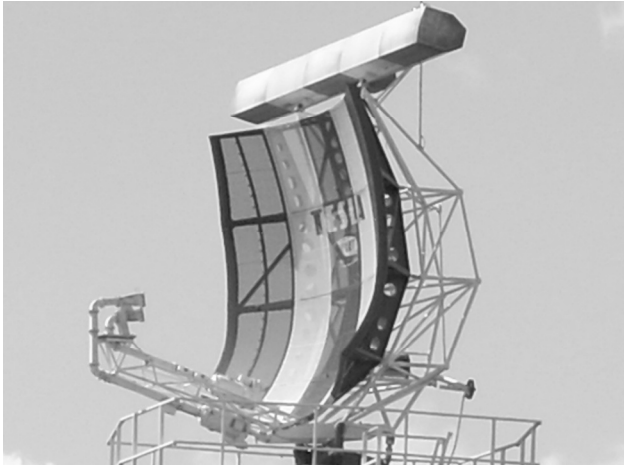
Fig. 2. The RL-41 antenna - doubly curved reflector with two independent pyramidal horns and SSR antenna above.
