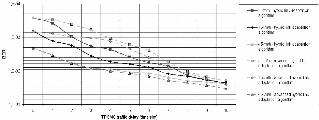
Fig. 4. Average L1 data BERs at various MS velocity and TPCM traffic delay.
