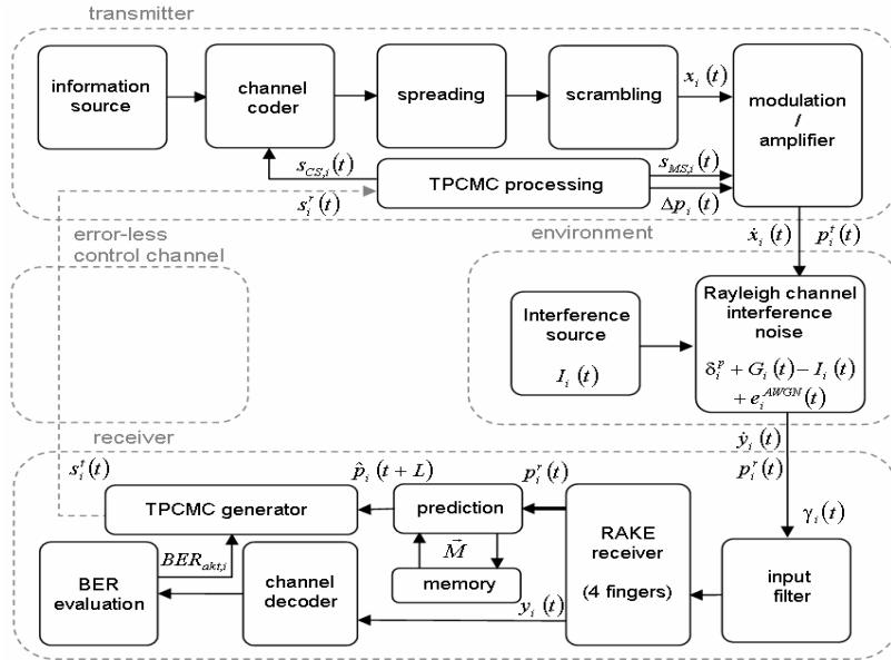
Fig. 3. WCDMA based transmitter / receiver block diagram.
