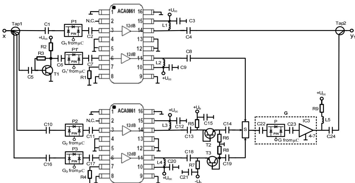
Fig.4. Predistorter electrical circuit diagram.
