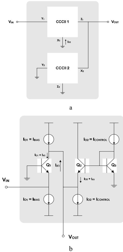
**Fig. 1.** New CCCII-based Low-Noise amplifiers (a) Guiding principle; (b) Final transistor-level diagram.
