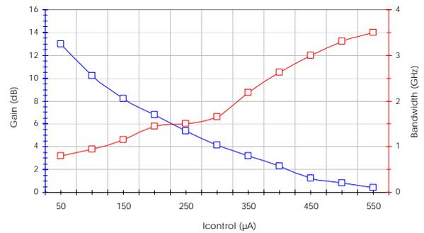
Fig. 4. Gain and bandwidth of the single-ended LNA at  $V_{DC} = \pm 1.5$  V and  $I_{BIAS} = 450$  μA.
