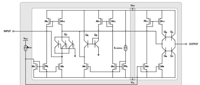
Fig. 2. Complete transistor-level description of a single-ended LNA based on the new principle.
