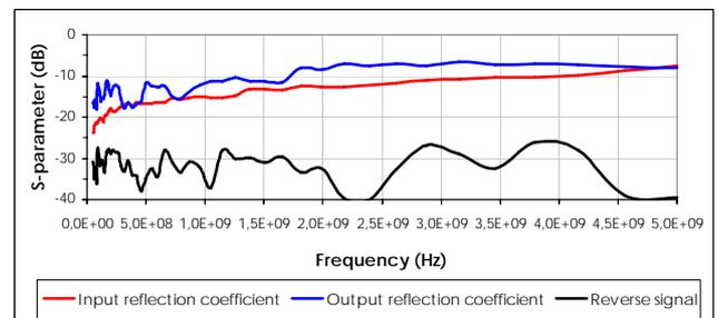
Fig. 5. S-parameters of the single-ended LNA, for gain = 6dB; at  $V_{DC} = \pm 1.5$  V and  $I_{BIAS} = 450$  μA.
