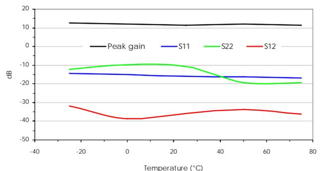
Fig. 7. S-parameters of the single-ended LNA, versus temperature, for gain = 10 dB; at  $V_{DC} = \pm 1.5$  V.
