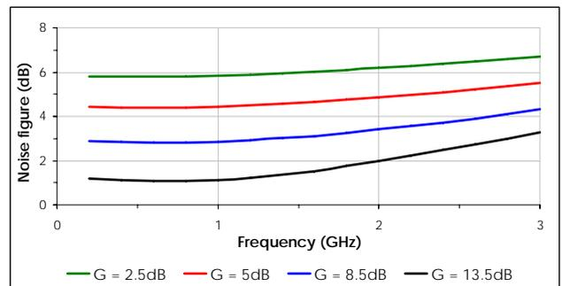
Fig. 6. Noise figure profiles for the single-ended LNA.
