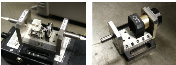
Fig. 9. The beam splitter assembly with polarizer and integrated collimators (left) and orthoconjugate retroreflector (right).
