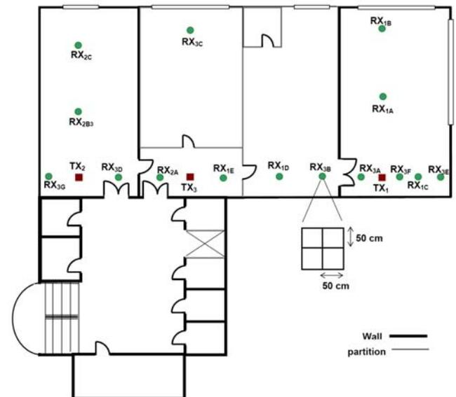
Fig. 3. Plan of the measurement environment with different Tx and Rx locations.
