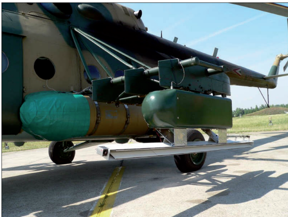
Fig. 13. SLAR equipment on a helicopter.
