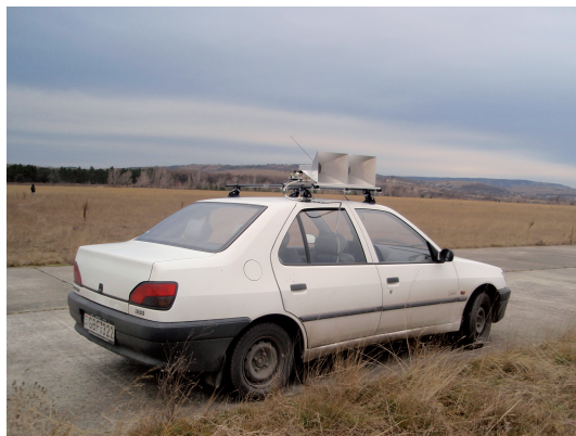
Fig. 17. SAR equipment on a car.
