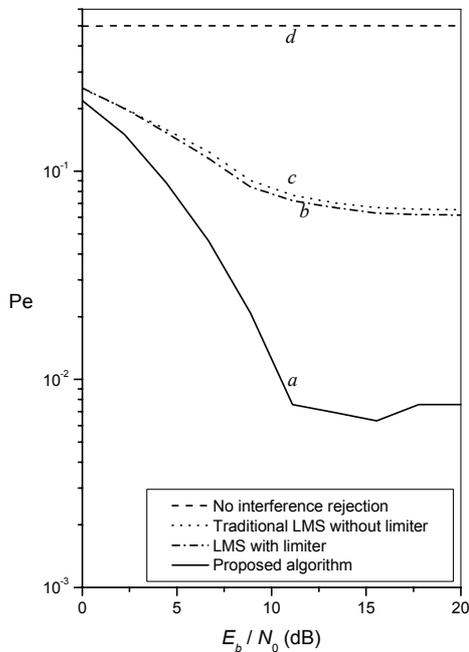
Fig. 3. Error probability as a function of signal to noise ratio.
