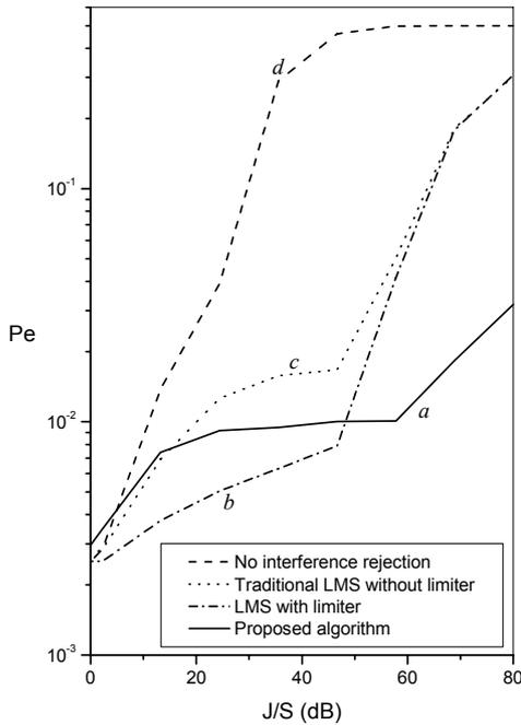
Fig. 2. Error probability as a function of interference to signal ratio.
