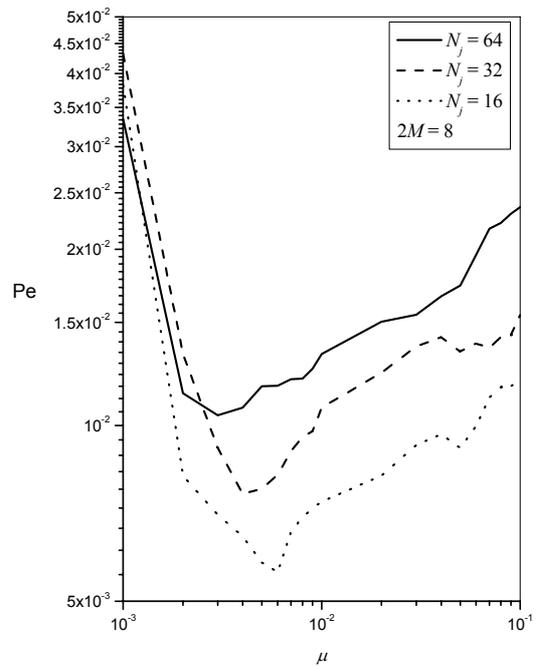
Fig. 4. Error probability as a function of LMS adaptation factor  $\mu$ .
