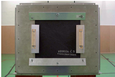
Fig. 4. Transmission measurements – Shielded box with sample 7 attached.
