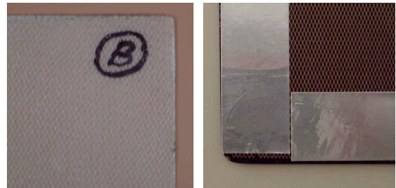
Fig. 1. Measured sample B (left) and sample 7 (right). Only a small part of sample is shown to emphasize nature of a printed metal grid.
