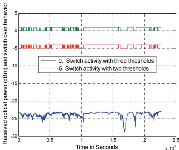
Fig. 6. Snow event of 28-11-2005 and behavior of wireless sensor network for selecting communication link [35].
