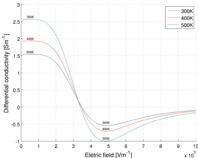
Fig. 2. Differential conductivity characteristics of the bulk GaAs at different temperatures.
