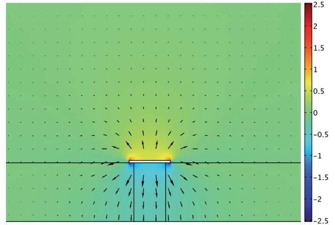
Fig. 6. The solution of Poisson equation. Surface: Electric field intensity,  $z$  component  $[\text{kVm}^{-1}]$  Arrow: Electric field intensity, transversal vector.
