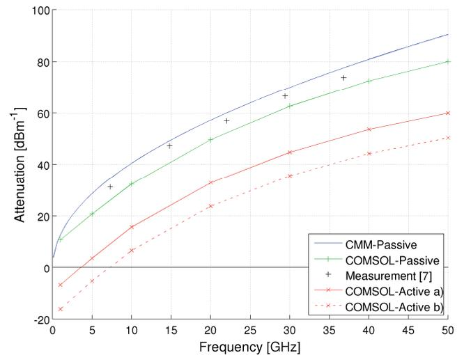
Fig. 3. Frequency response of the attenuation for passive and active microstrip line; a) HTC = 100 kWm<sup>-2</sup>K<sup>-1</sup>, b) HTC = 10 kWm<sup>-2</sup>K<sup>-1</sup>.
