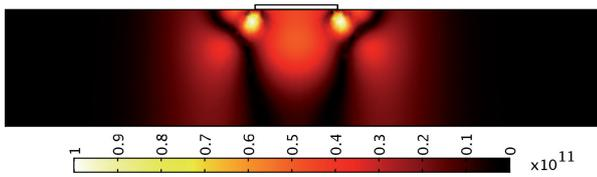
Fig. 4. Distribution of resistive heating  $[\text{Wm}^{-1}]$  inside the GaAs substrate uniformly doped by donors at concentration  $10^{19} \text{ m}^{-3}$ .
