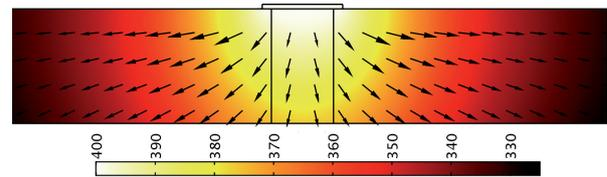
Fig. 7. Temperature distribution in continuous regime. Surface: temperature  $[\text{K}]$ . Arrow: Heat flux vector.
