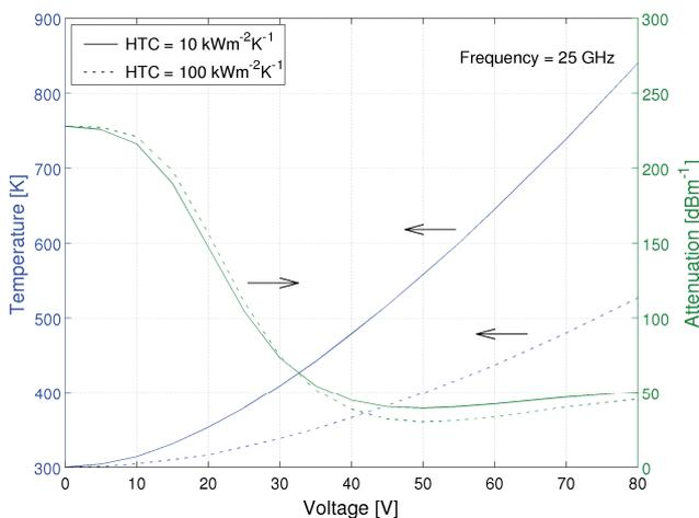
**Fig. 10.** The dependency of temperature and attenuation on applied bias voltage.
