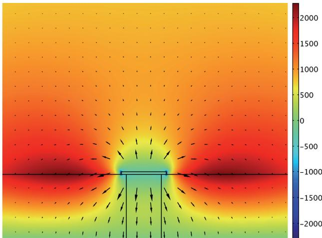
**Fig. 9.** Electric field intensity of the fundamental mode at 25 GHz. Surface: Electric field intensity, x component [ $\text{Vm}^{-1}$ ] Arrow: Electric field intensity, transversal vector.
