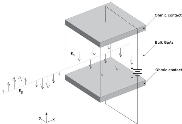
Fig. 1. Illustrative sketch of wave propagation in biased GaAs sample.
