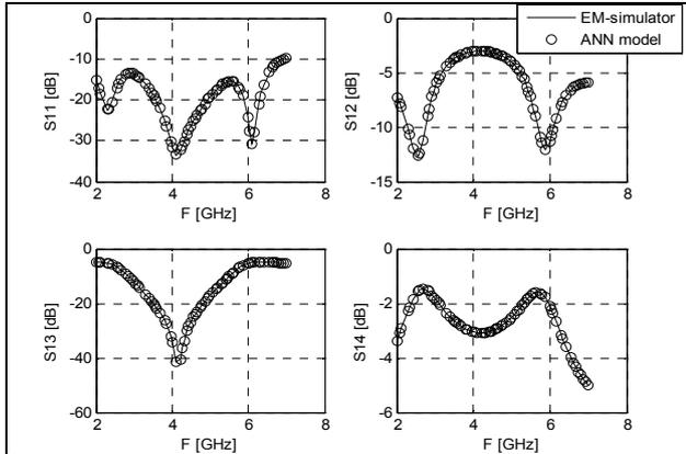
Fig. 4. Stripline type RHC ( $f_{cen} = 4.16$  GHz) scattering parameters: EM simulator vs. NN model.
