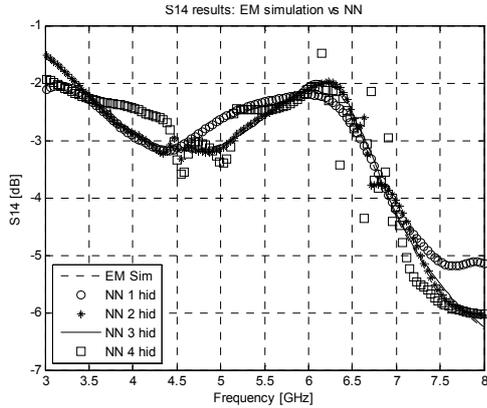
Fig. 7.  $S_{14}$  results: EM simulator vs. NN results for LM ( $f_{cen} = 4526$  MHz).
