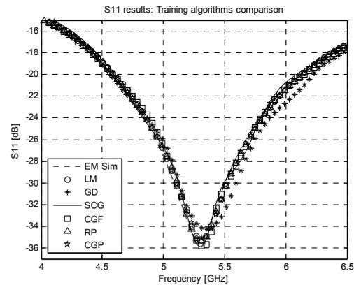
Fig. 8. Comparison of training algorithms for  $S_{11}$  ( $f_{cen} = 5269$  MHz).
