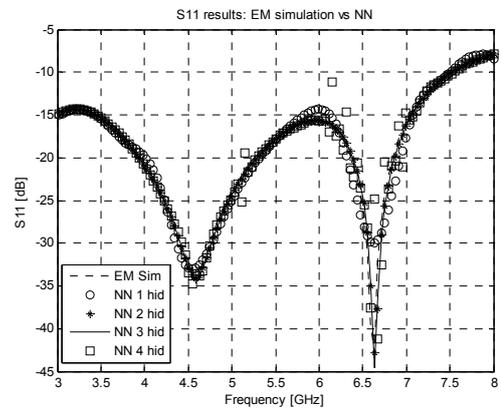
Fig. 5.  $S_{11}$  results: EM simulator vs. NN results for LM ( $f_{cen} = 4526$  MHz).
