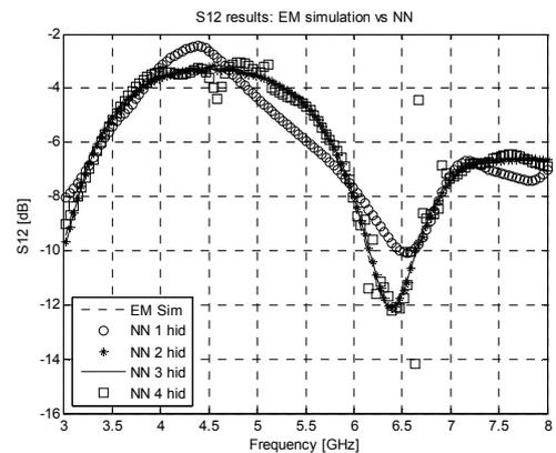
Fig. 6.  $S_{12}$  results: EM simulator vs. NN results for LM ( $f_{cen} = 4526$  MHz).
