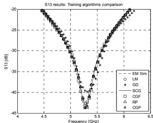
Fig. 10. Comparison of training algorithms for  $S_{13}$  ( $f_{cen} = 5269$  MHz)
