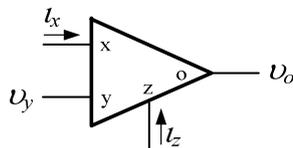
Fig. 1. Used notation for the CFOA.
