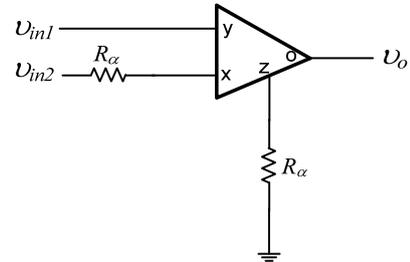
Fig. 3. CFOA based subtraction block.
