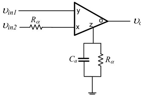
Fig. 2. CFOA based lossy integration-subtraction block.
