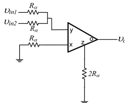
Fig. 4. CFOA based summation block.
