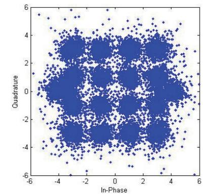
f) PO channel and portable reception scenario, MER = 17.5 dB; BER<sub>1</sub> = 3.8 · 10<sup>-3</sup>; BER<sub>2</sub> = 2.1 · 10<sup>-6</sup>
