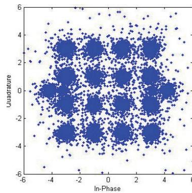
e) PI channel and portable reception scenario, MER = 18.4 dB; BER<sub>1</sub> = 2.5 · 10<sup>-3</sup>; BER<sub>2</sub> < 1 · 10<sup>-6</sup>
