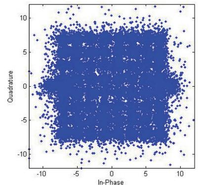
c) RL20 ANX B channel and fixed reception scenario, MER = 15.7 dB; BER<sub>1</sub> = 2.3 · 10<sup>-2</sup>; BER<sub>2</sub> = 2.4 · 10<sup>-3</sup>
