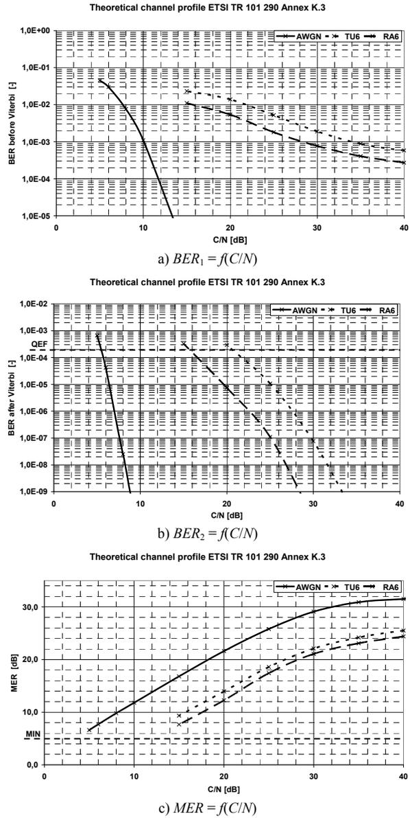
Fig. 6. Measurement: Mobile reception scenario (QPSK, 2k mode, code rate 2/3 and GI 1/16) and DVB-T/H performance in typical transmission channel profiles.
