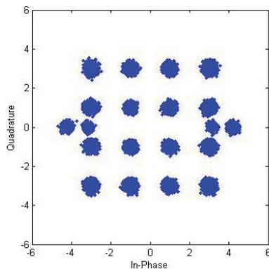
d) AWGN channel and portable reception scenario, MER = 25.0 dB; BER<sub>1</sub> < 1 · 10<sup>-6</sup>; BER<sub>2</sub> < 1 · 10<sup>-6</sup>
