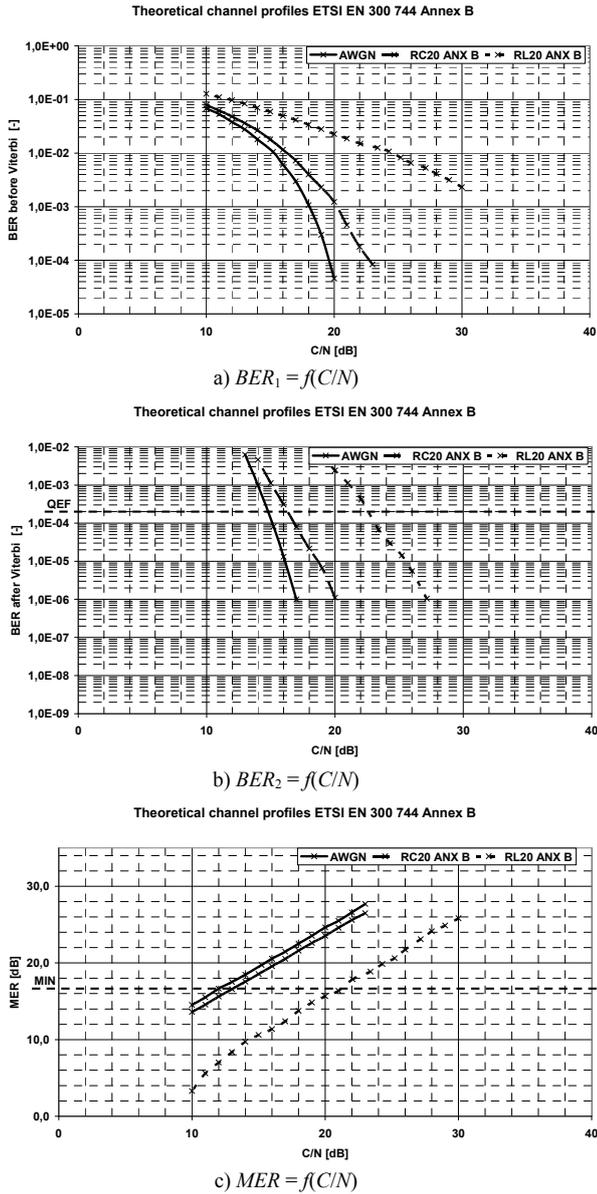
**Fig. 1.** Simulation: Fixed reception scenario (64-QAM, 8k mode, code rate 2/3 and GI 1/8) and DVB-T/H performance in typical transmission channel profiles.
