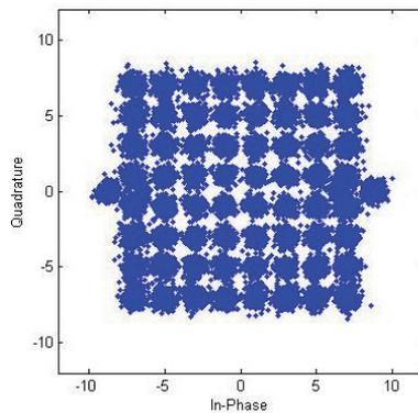
b) RC20 ANX B channel and fixed reception scenario, MER = 23.5 dB; BER<sub>1</sub> = 1.2 · 10<sup>-3</sup>; BER<sub>2</sub> = 1.1 · 10<sup>-6</sup>
