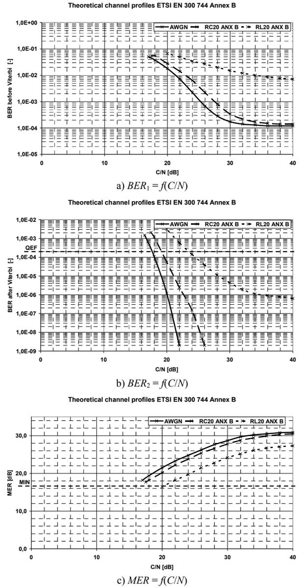
**Fig. 2.** Measurement: Fixed reception scenario (64-QAM, 8k mode, code rate 2/3 and GI 1/8) and DVB-T/H performance in typical transmission channel profiles.
