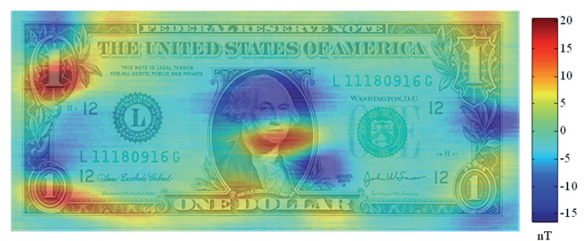
Fig. 8. Mapped gradient field of a 1-USD banknote, as measured 5 mm above the plane.
