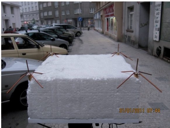
Fig. 4. Receive antenna diversity arrangement at street level.
