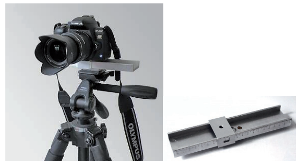
Fig. 10. Sliding attachment on a tripod was used to capture stereoscopic pairs.
