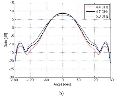
**Fig. 9.** Radiation patterns of the E-shaped stacked-patch antenna with washer: E-field (a), H-field (b).
