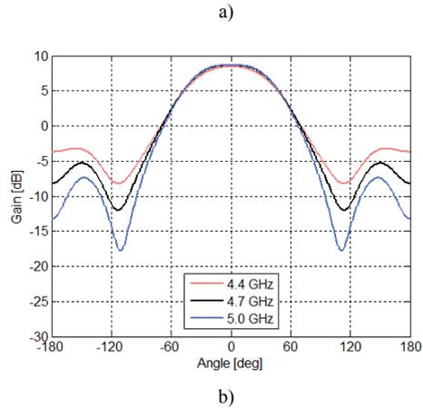
Fig. 3. Radiation patterns of the aperture-fed antenna: E-field (a), H-field (b).
