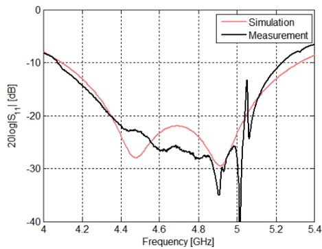
**Fig. 22.** Reflection coefficient of the array with U-slot patches.
