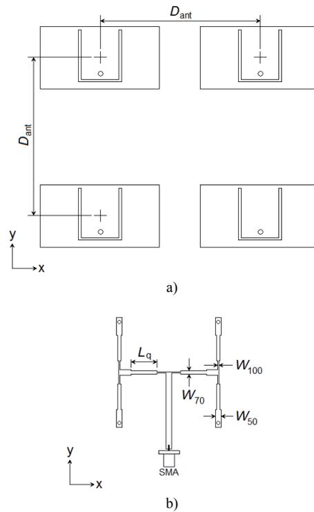
Fig. 20. Schematics of the array with U-slot patches: top view (a), feeding network (b).
