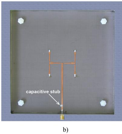
**Fig. 21.** Photograph of the fabricated array with U-slot patches: top view - the radome was removed (a), feeding network - the top shield of the metallic box was removed (b).
