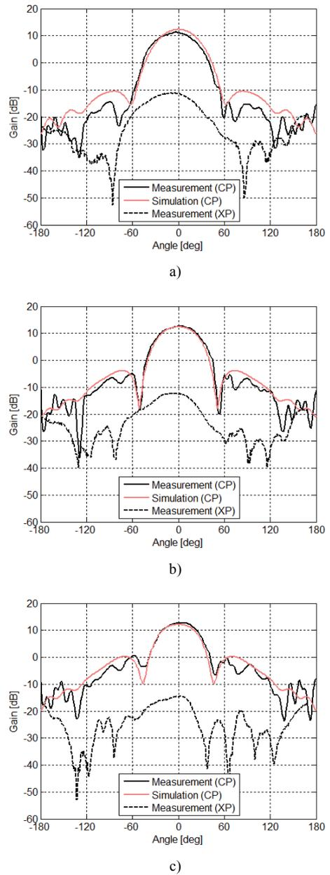
**Fig. 24.** Radiation patterns (H-field) of the array with U-slot patches: 4.4 GHz (a), 4.7 GHz (b), 5.0 GHz (c).
