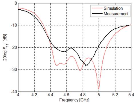
**Fig. 16.** Reflection coefficient of the array with E-shaped patches and washer.
