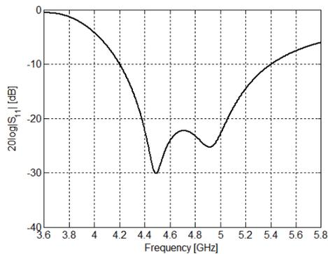
Fig. 11. Reflection coefficient of the U-slot patch antenna.
