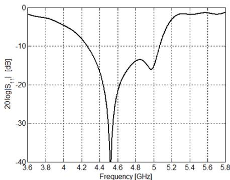
Fig. 5. Reflection coefficient of the stacked-patch antenna.
