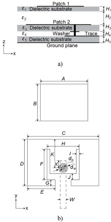
**Fig. 7.** Schematics of the E-shaped stacked-patch antenna with washer: side view (a), top view – the upper patch and the lower patch (b).
