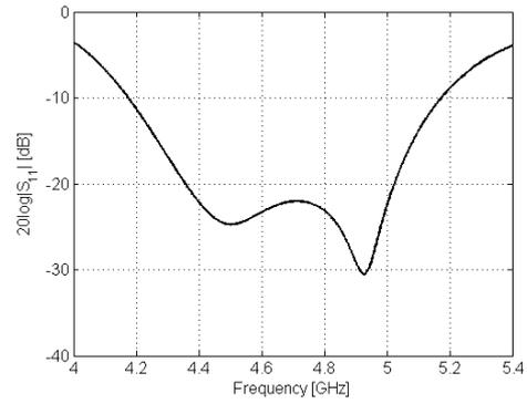
**Fig. 8.** Reflection coefficient of the E-shaped stacked-patch antenna with washer.
