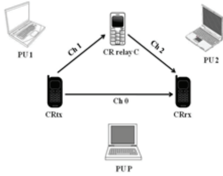
Fig.1. Cooperative cognitive radio network with relay.
