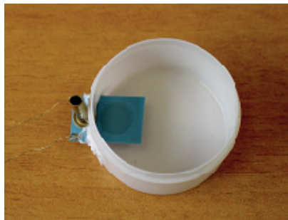
Fig. 4. The CCPS mounted in the plastic pot to prevent contact of the electrical contacts with water during the experimentation.
