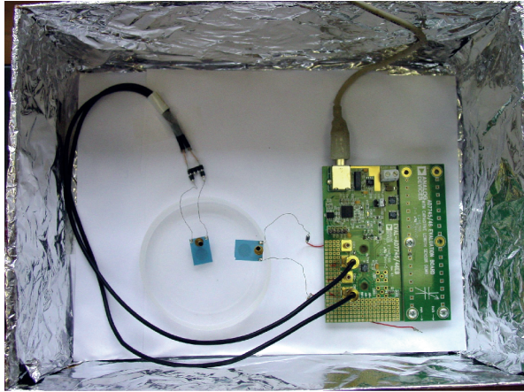
Fig. 3. Experimental set-up with AD7746 evaluation board used for evaluation of the effect of the humidity and moisture on the CCPS.
