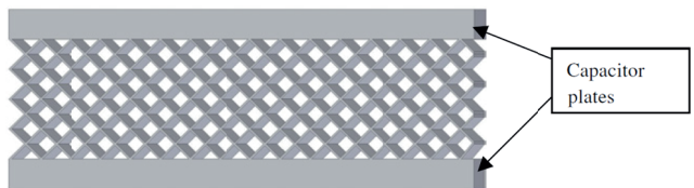
Fig. 4. Honeycomb-type variable capacitor [7].
