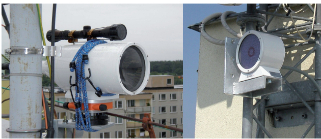
Fig. 1. Scintec Boundary Layer Scintillometer BLS450, LED transmitter – right, receiver – left.
