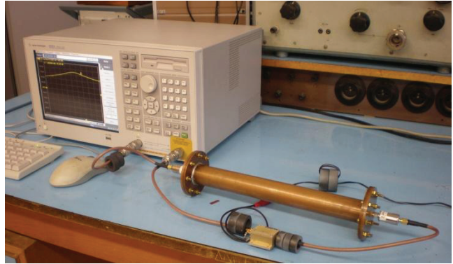
Fig. 4. Experimental setup for the measurement of resistance.
