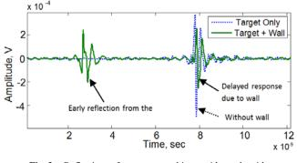
Fig. 3. Reflections from target object with and without obstruction.
