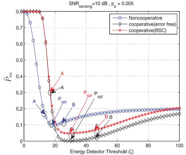
Fig. 3. The modified miss-detection probability  $\tilde{P}_m$  for different spectrum sensing configurations versus  $\zeta$ . Solutions of the optimization problem (11) are indicated by  $P_{opt}$ .
