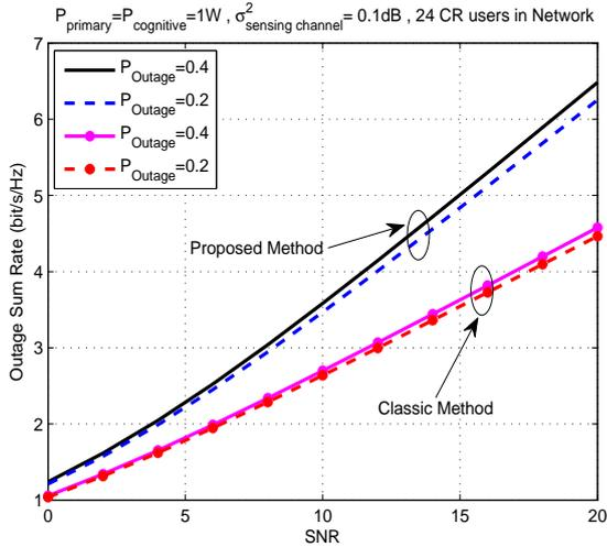
Fig. 7. Primary achievable outage information rates over the BSC reporting channel versus the SNR for the proposed spectrum sensing method with 24 cognitive user cooperating in the sensing process.
