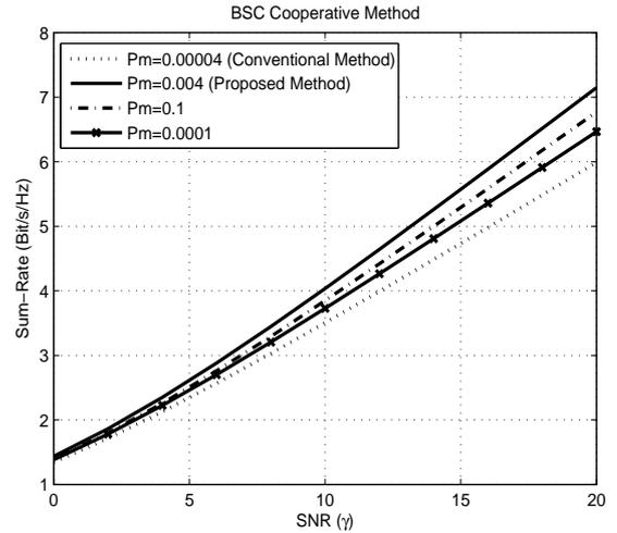
**Fig. 5.** Total achievable information rates over the BSC reporting channel versus the SNR for different spectrum sensing methods with 12 cognitive user cooperating in the sensing process.
