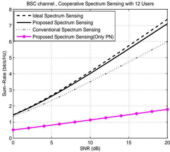
**Fig. 4.** Total achievable information rates over the BSC reporting channel versus the SNR for different spectrum sensing methods with 12 cognitive user cooperating in the sensing method.
