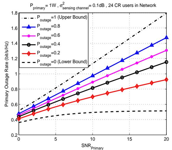
**Fig. 6.** Achievable outage sum-rates over the error-free reporting channel versus the SNR for proposed spectrum sensing method with 24 cognitive user cooperating in the sensing process.
