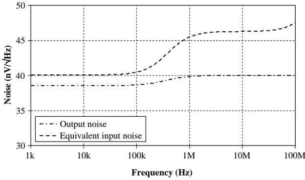
Fig. 6. Input and output noise variations versus frequency.
