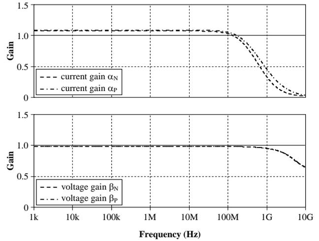
Fig. 3. Characteristics of the proposed DCCII implementation.
