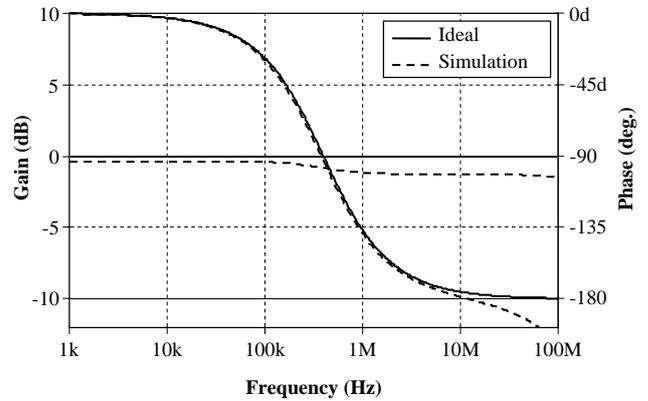
Fig. 4. Ideal and simulated gain and phase responses for the presented first-order all-pass filter.
