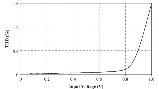
Fig. 5. THD variations versus amplitudes of the applied sinusoidal input voltages at  $f_0 \approx 398$  kHz.
