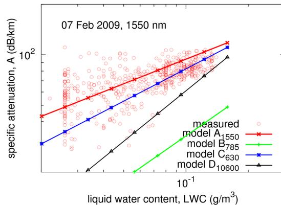
Fig. 5. Comparison of the models with measured data, 7 February 2009, wavelength 1550 nm.
