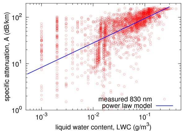
Fig. 2. Optical attenuation and LWC measured in Prague, January - May 2009, wavelength 830 nm; fitted power law model (3).
