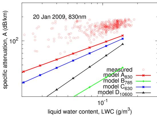
Fig. 7. Comparison of the models with measured data, 20-21 January 2009, wavelength 830 nm.
