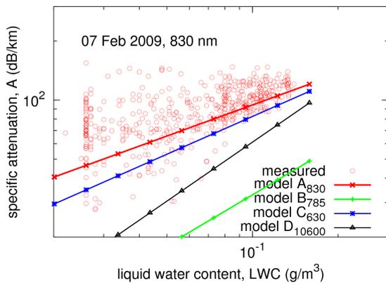
Fig. 8. Comparison of the models with measured data, 7 February 2009, wavelength 830 nm.
