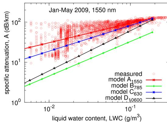
Fig. 6. Comparison of the models with measured data, January-May 2009, wavelength 1550 nm.
