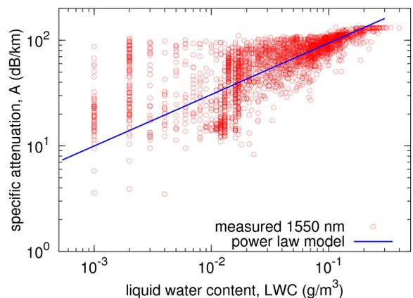
Fig. 3. Optical attenuation and LWC measured in Prague, January - May 2009, wavelength 1550 nm; fitted power law model (4).
