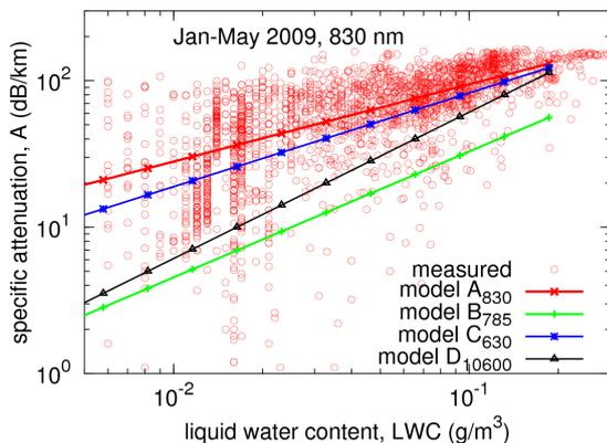
Fig. 9. Comparison of the models with measured data, January-May 2009, wavelength 830 nm.
