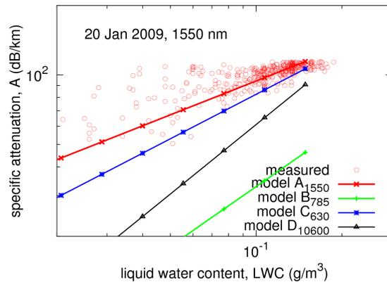
Fig. 4. Comparison of the models with measured data, 20-21 January 2009, wavelength 1550 nm.
