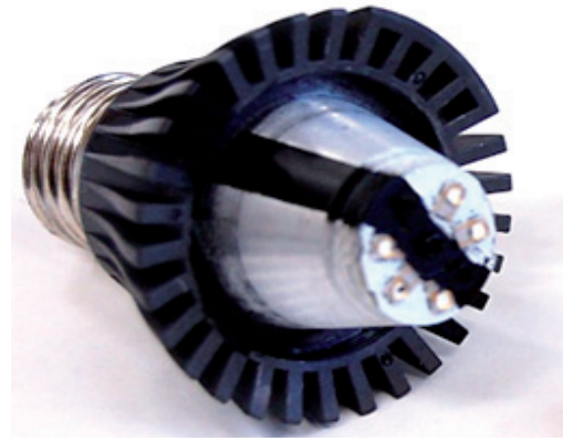
Fig. 5. SSL lamp components with black strip used for IR measurement.
