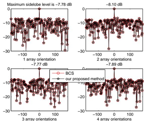
Fig. 3. Optimal beam pattern of different element number array by using “BCS inversion algorithm [11]” vs. “Our method”.
