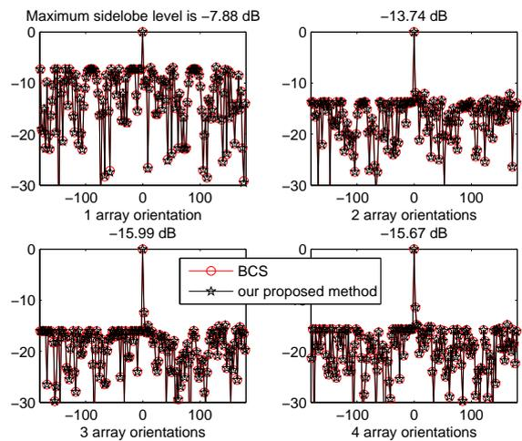
Fig. 2. “Reference beam pattern of a 23(24)-element array by using BCS inversion algorithm[11]” vs. “Our beam pattern of a 23-element array”.
