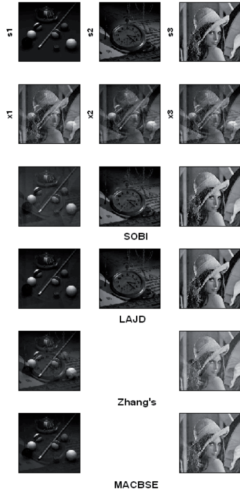
Fig. 2. Simulation results for mixtures of three 128 \times 128 image signals. From top to bottom, the original image sources 1-3, the mixed image mixtures 1-3, the three separated images using the SOBI algorithm, the three separated images using the proposed LAJD algorithm, the extracted two images using the Zhang's algorithm and the extracted two images using the MACBSE algorithm.
