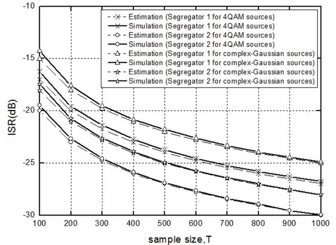
**Fig. 1.** *ISR* versus sample size for Segregator 1 and 2 when  $n = 20, r = 1$ .
