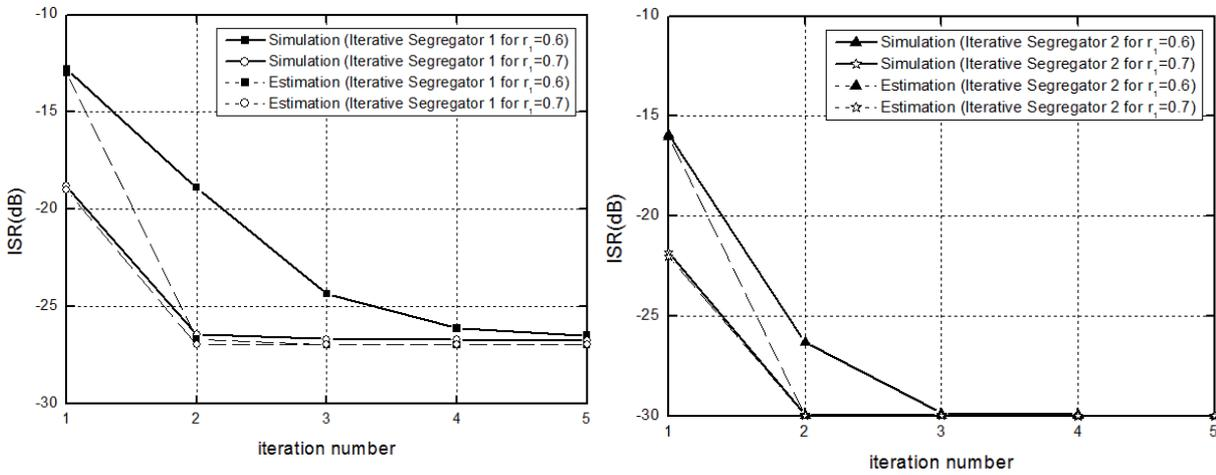
Fig. 4.  $ISR$  of Iterative Segregator 1 and 2 for different initial correct support estimation ratios when  $n = 10$  4QAM sources and  $T = 1000$  samples are adopted.
