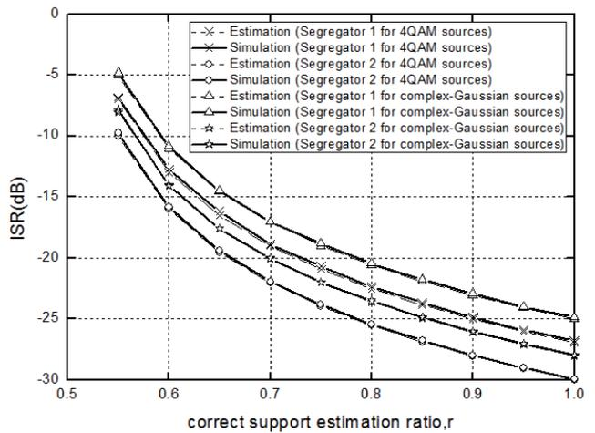
**Fig. 2.** *ISR* versus correct support estimation ratio for Segregator 1 and 2 when  $n = 20$  and  $T = 1000$ .
