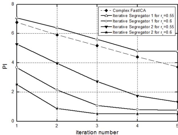
Fig. 5. Performance index ( $PI$ ) among Complex FastICA, Iterative Segregator 1 and 2 when  $n = 10$  4QAM sources and  $T = 1000$  samples are adopted.
