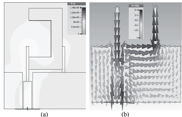
Fig. 6. (a) Simulated volume electric field distributions and (b) surface current at 4 GHz of the optimized CP DRA.
