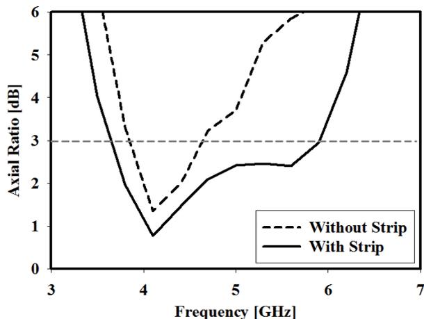
Fig. 4. Comparison between simulated AR of the CPDRA with and without the grounded narrow strip.
