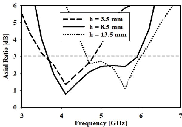
Fig. 3. Simulated AR of the CPDRA with different values of  $h$ .
