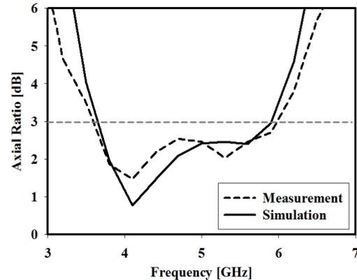
Fig. 8. Measured and simulated AR of the CPDRA.
