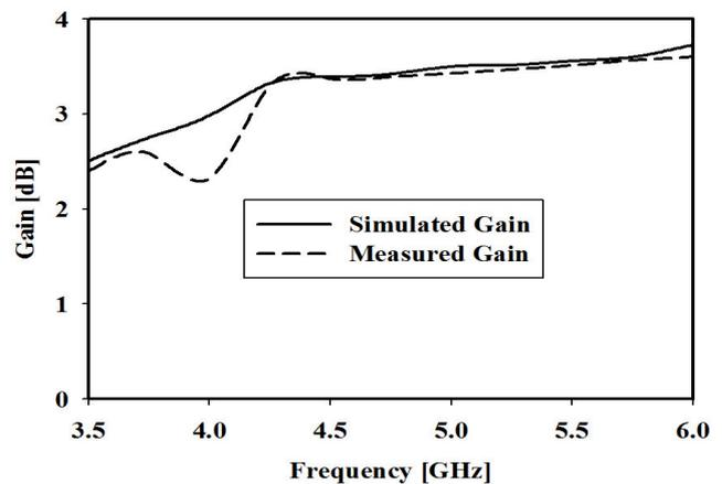
Fig. 10. Measured and simulated gain of the proposed CPDRA.
