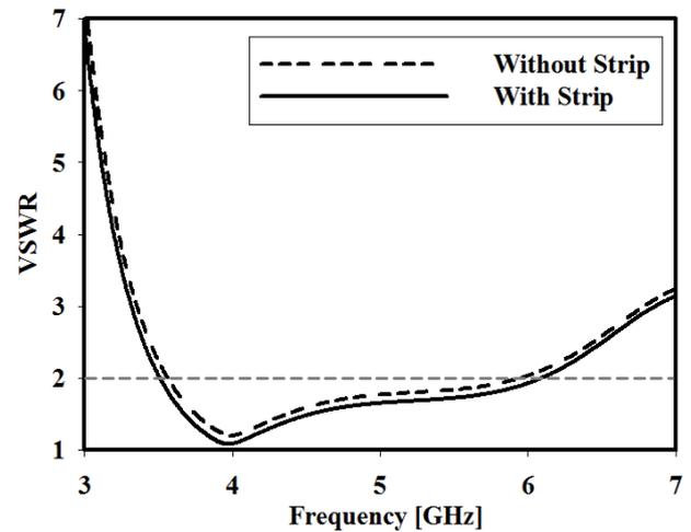
Fig. 5. Comparison between simulated VSWR of the antenna with and without grounded narrow strip.
