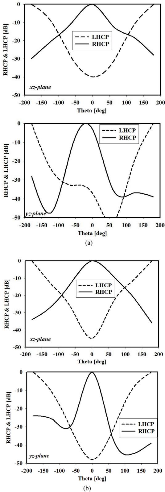
Fig. 11. Radiation patterns (RHCP and LHCP) of the realized antenna at: (a) 4 GHz and (b) 5.2 GHz for xz-plane and yz-plane.
