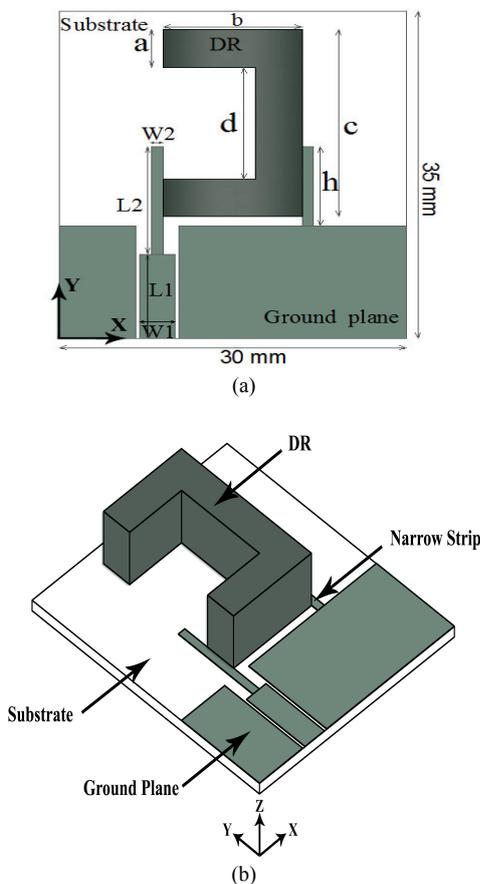
**Fig. 1.** (a) Top view and (b) 3D view of the proposed CPDRA.
