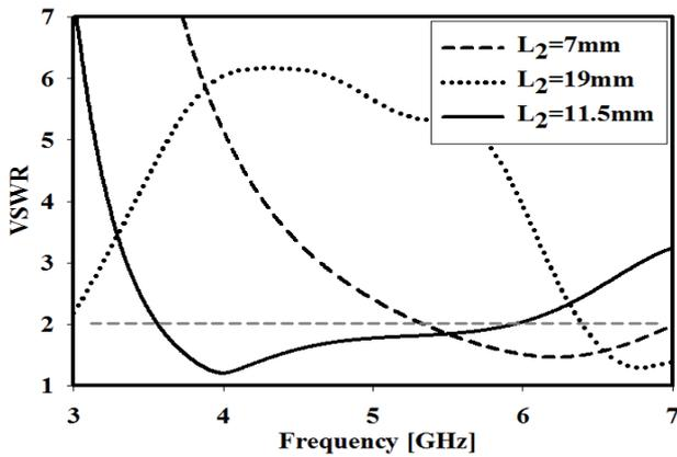
Fig. 2. Simulated VSWR of the CPDRA with different values of  $L_2$ .
