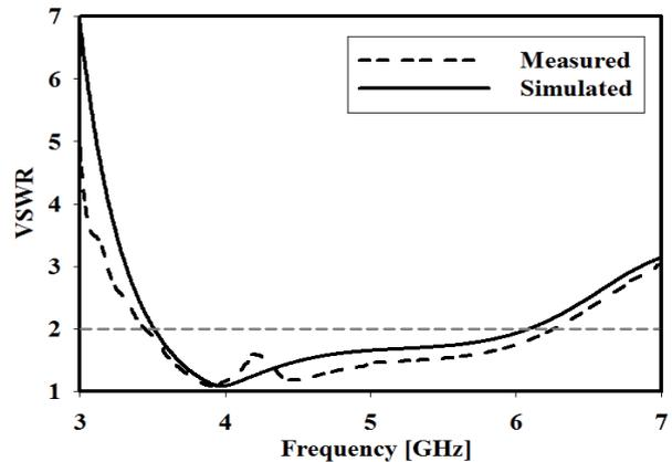
Fig. 9. Measured and simulated VSWR of the CPDRA.
