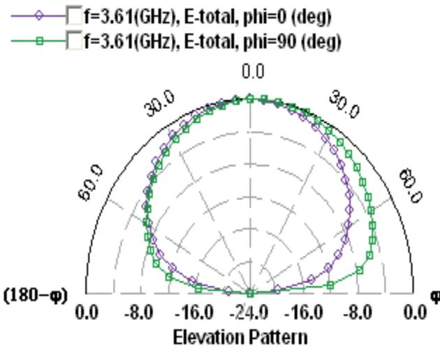
Fig. 13. (c) Two dimensional E and H plane elevation patterns at frequency 3.61 GHz.
