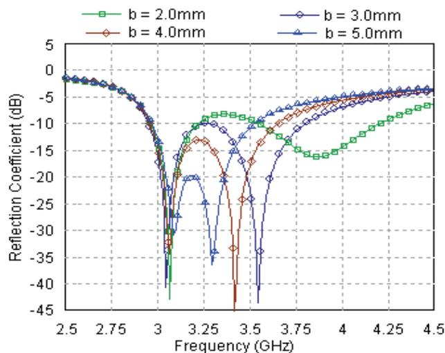
**Fig. 6.** Simulated reflection coefficient of the proposed antenna with different *b* values (with constant *h<sub>f</sub>* = 3.0 mm).
