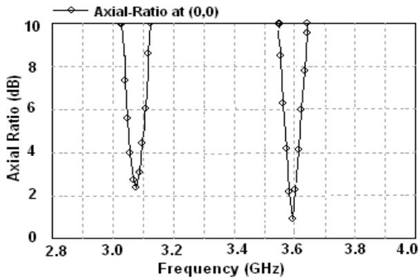
Fig. 9. Measured axial ratio variation with frequency for the multi-layered modified rectangular patch antenna.
