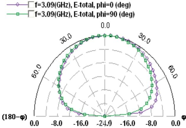
Fig. 13. (b) Two dimensional E and H plane elevation patterns at frequency 3.09 GHz.
