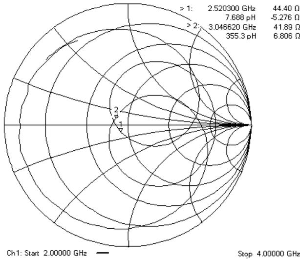
Fig. 3. Measured variation of input impedance for the single layer modified rectangular patch antenna.
