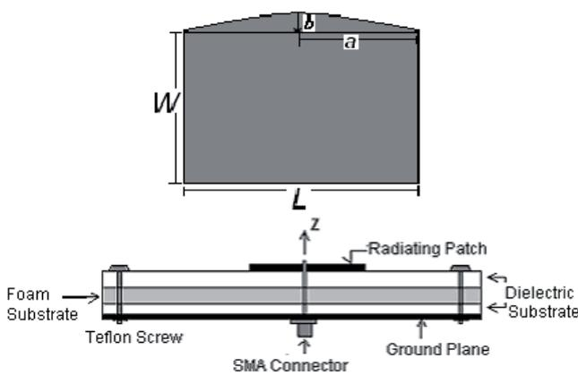
Fig. 4. Geometry of the modified rectangular patch antenna with protruded curved edge designed on multilayered structure.
