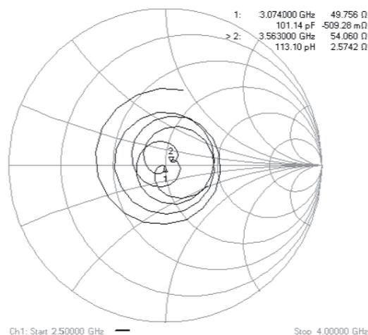
**Fig. 8.** Measured input impedance variation of the multi-layered modified rectangular patch antenna with frequency.
