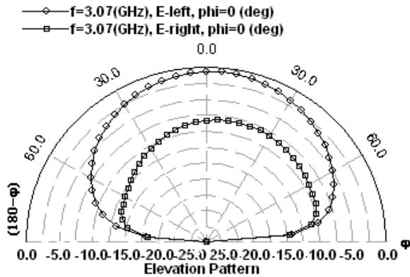
Fig. 10. E plane left and right circularly polarized patterns at 3.07 GHz for the proposed antenna.
