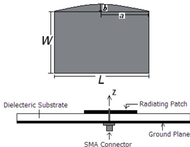
Fig. 1. Top and side view of the designed single layer modified rectangular patch antenna with feed arrangement.
