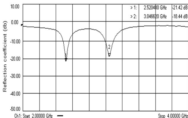
Fig. 2. Measured variation of reflection coefficient with frequency for the single layer modified rectangular patch antenna.
