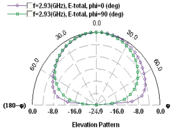
Fig. 13. (a) Two dimensional E and H plane elevation patterns at frequency 2.93 GHz.
