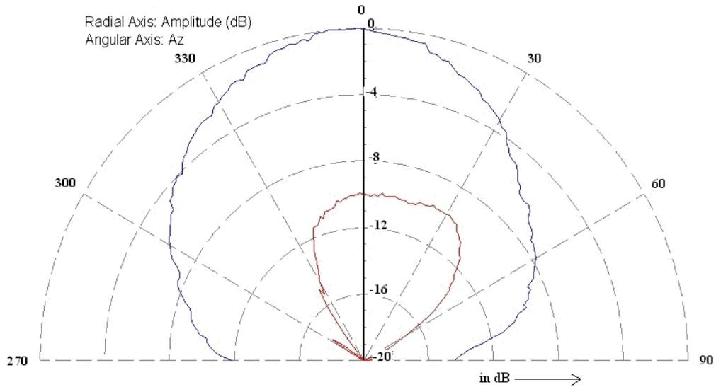
Fig. 14. (b) Measured E plane co and cross-polar radiation patterns at frequency 3.55 GHz.
