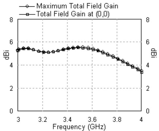
Fig. 13. Variation of the directive gain with frequency for the proposed antenna.
