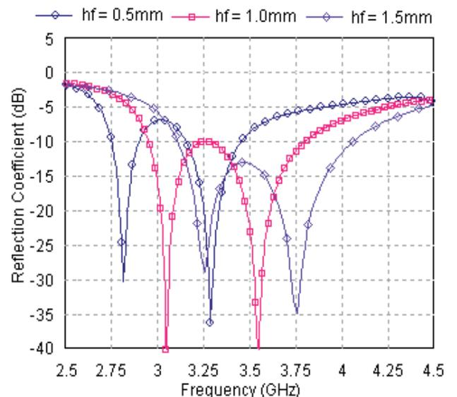
Fig. 5. Simulated reflection coefficient of the proposed antenna with different  $h_f$  values (with constant  $b = 3.0$  mm).
