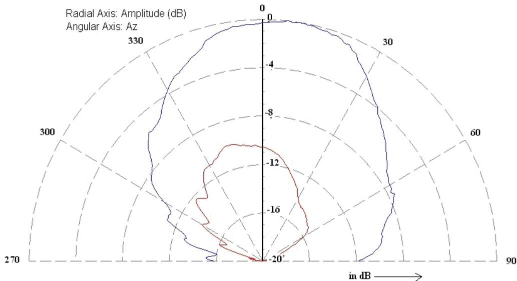
Fig. 14. (a) Measured E plane co and cross-polar radiation patterns at frequency 3.07 GHz.
