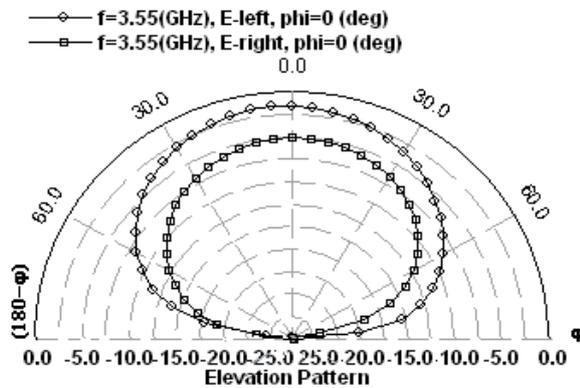
Fig. 11. E plane left and right circularly polarized patterns at 3.55 GHz for the proposed antenna.
