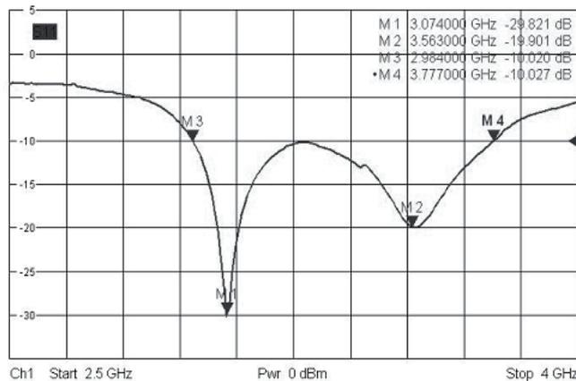
**Fig. 7.** Measured *S*<sub>11</sub> variation of the multi-layered modified rectangular patch antenna with frequency.
