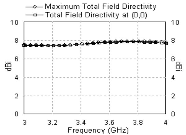
Fig. 12. Variation of the total field directivity with frequency for the proposed antenna.
