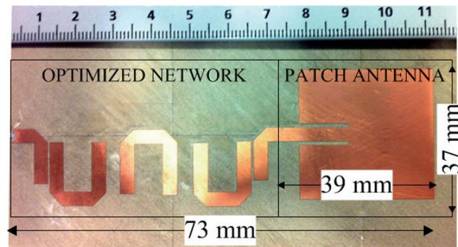
Fig. 11. Filtenna prototype fabricated in microstrip technology.
