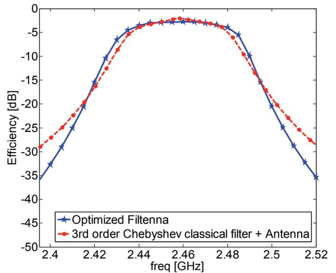
Fig. 7. Efficiency of the filtenna in blue solid line and efficiency of a 3<sup>rd</sup> order Chebyshev filter ( $BW = 50$  MHz &  $RL = 15$  dB) + antenna in red dashed line.
