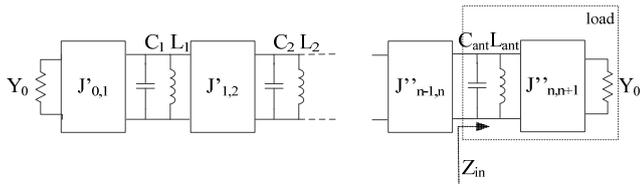
**Fig. 3.** The network from Fig. 2 where all the impedance inverters have been scaled in order to obtain an ideal filter response.
