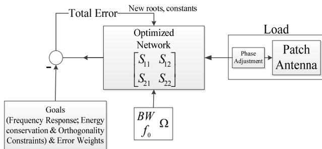
Fig. 5. Flowchart describing the optimization procedure.
