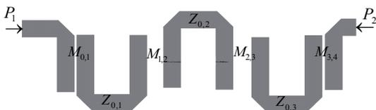
Fig. 9. Optimized network designed in microstrip technology.
