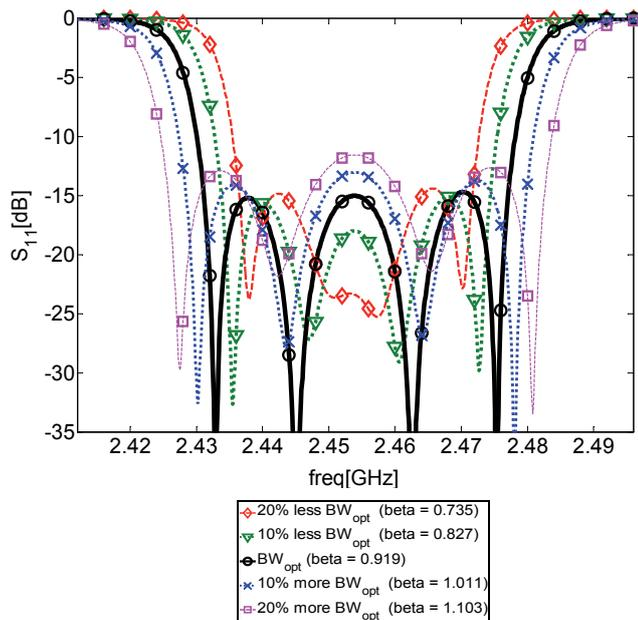
**Fig. 4.** Return Losses of a 4-pole filtenna vs.  $\beta$  for a given RLC antenna.
