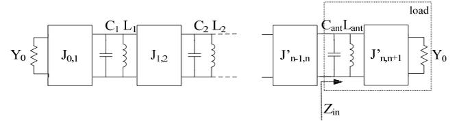
Fig. 2. The network from Fig. 1 where the last filter stage is framed representing the load antenna, after scaling the last impedance.
