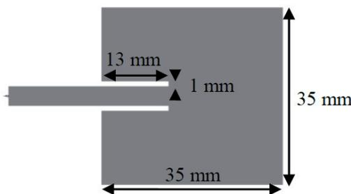
Fig. 6. Microstrip patch antenna.
