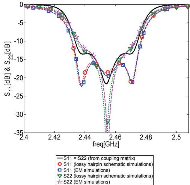
Fig. 10. 3<sup>rd</sup> order 2-port network placed before the antenna.  $S_{11}$  &  $S_{22}$  parameters.
