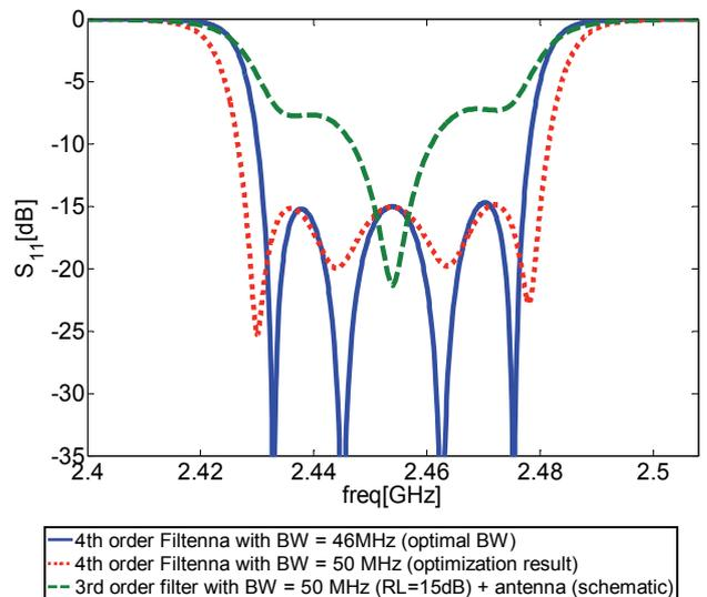
Fig. 8. 50 MHz bandwidth optimization – red dotted line – vs. Optimal BW response found for our microstrip patch antenna ( $BW = 46$  MHz) – blue solid line – vs. 3<sup>rd</sup> order filter ( $BW = 50$  MHz &  $RL = 15$  dB) + Antenna.
