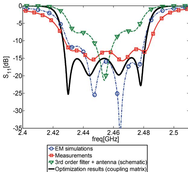
Fig. 12. 4<sup>th</sup> order filtenna (optimization results & EM simulations & measurements) vs 3<sup>rd</sup> order filter + antenna.
