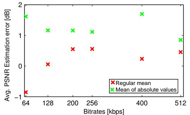
Fig. 7. Average estimation error in comparison to used bitrates.
