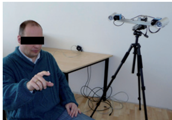
Fig. 1. Motion capture camera system during finger-tapping test measurement.
