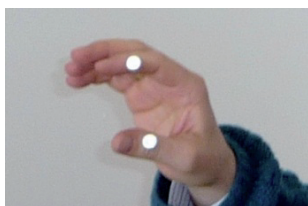
Fig. 2. Hand with passive markers placed on the first knuckles of the forefinger and thumb.
