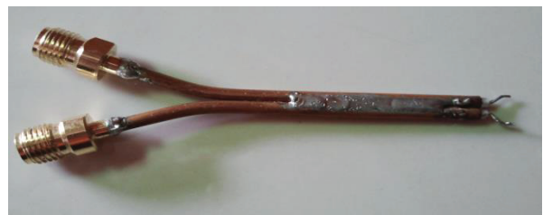
Fig. 3. Prototype of test fixture.
