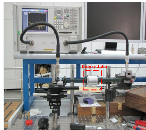
Fig. 8. Measurement setup of the fabricated rotary joint.
