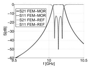
**Fig. 6.** *S*-characteristics of the waveguide filter with inhomogeneity in the *z* direction obtained using standard FEM and FEM-MOR for  $\phi_{1...4} = [-30^\circ, -28^\circ, 28^\circ, 30^\circ]$ .
