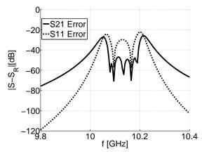
**Fig. 7.** Absolute error for  $S_{11}$  and  $S_{21}$  values computed using a FEM and FEM-MOR for  $\phi_{1...4} = [-30^{\circ}, -28^{\circ}, 28^{\circ}, 30^{\circ}]$ .
