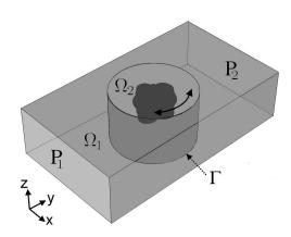
Fig. 2. A waveguide structure with an arbitrary rotatable discontinuity closed in the cylindrical subdomain  $\Omega_2$ , separated from the rest of the computational domain by means of the surface  $\Gamma$ . Surfaces  $P_1$  and  $P_2$  are the excitation ports.
