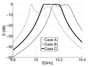
**Fig. 9.**  $S_{21}$ -characteristics of the waveguide filter obtained using FEM-MOR for 3 cases of  $\phi_{1...4}$ :  $A[-10^{\circ}, -80^{\circ}, 80^{\circ}, 10^{\circ}]$ ,  $B[50^{\circ}, 0^{\circ}, 0^{\circ}, -50^{\circ}]$  and  $C[-30^{\circ}, -28^{\circ}, 28^{\circ}, 30^{\circ}]$ .
