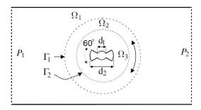
Fig. 3. Elevation view of the 3D WR-90 waveguide structure with centrally placed rotatable bow-tie tuning element.  $d_1=1.5\,\mathrm{mm},\ d_2=5\,\mathrm{mm},\ \mathrm{length}=40\,\mathrm{mm},\ \mathrm{width}=22.86\,\mathrm{mm},\ \mathrm{height}$  of the waveguide =  $10.16\,\mathrm{mm},\ \mathrm{height}$  of the bow-tie =  $9.16\,\mathrm{mm},\ \mathrm{diameter}$  of  $\Gamma_1=9\,\mathrm{mm}$  and diameter of  $\Gamma_2=8\,\mathrm{mm},\ \mathrm{rotation}$  angle of  $\Omega_3$ :  $\phi=0.$
