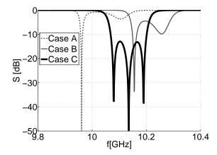
**Fig. 8.**  $S_{11}$ -characteristics of the waveguide filter obtained using FEM-MOR for 3 cases of  $\phi_{1...4}$ :  $A[-10^{\circ}, -80^{\circ}, 80^{\circ}, 10^{\circ}], B[50^{\circ}, 0^{\circ}, 0^{\circ}, -50^{\circ}]$  and  $C[-30^{\circ}, -28^{\circ}, 28^{\circ}, 30^{\circ}].$
